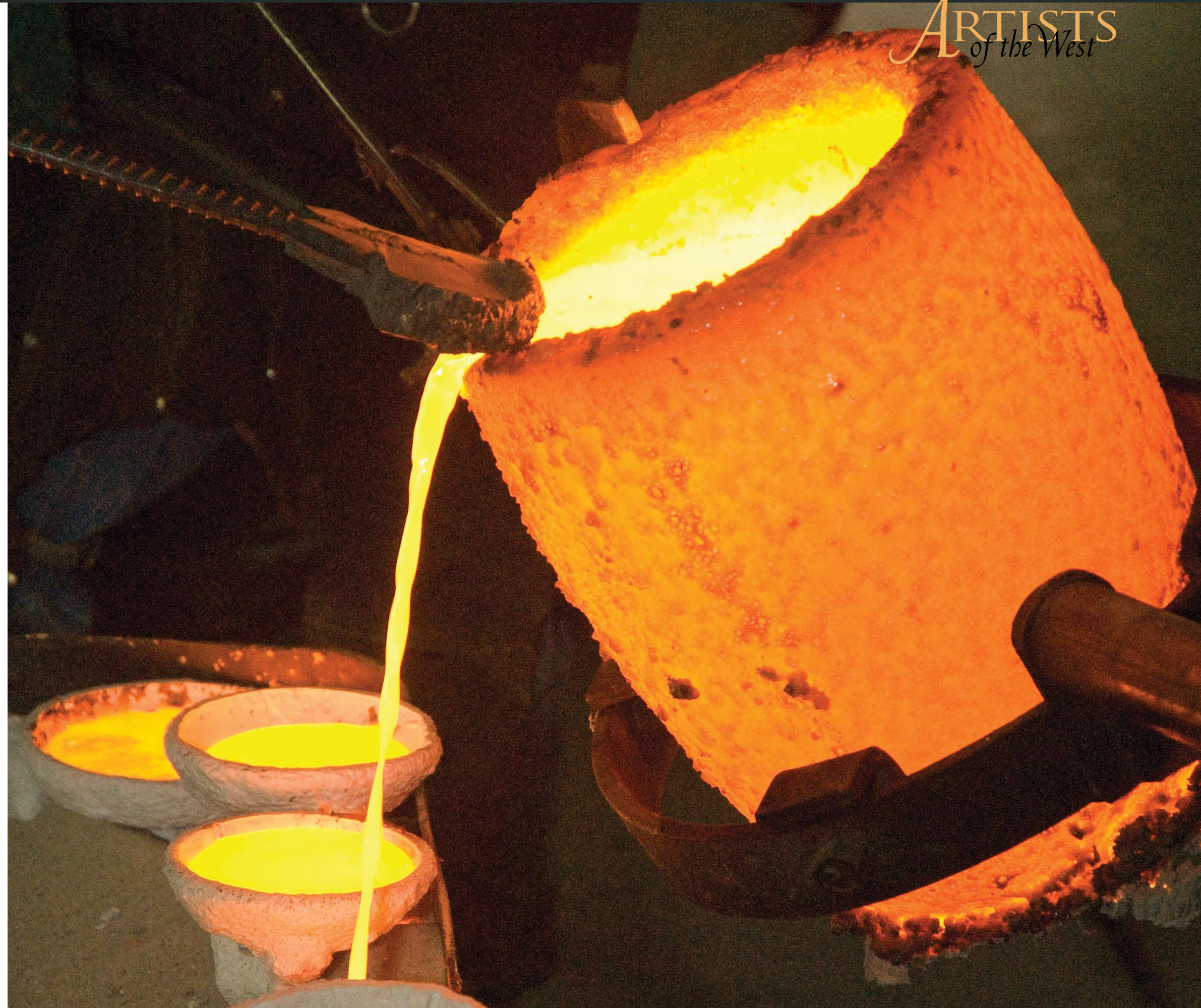
Above: Foundry owner and sculptor, Jack Muir in the gallery at his foundry Right: The molten bronze is carefully poured into the molds in the sand trough.
